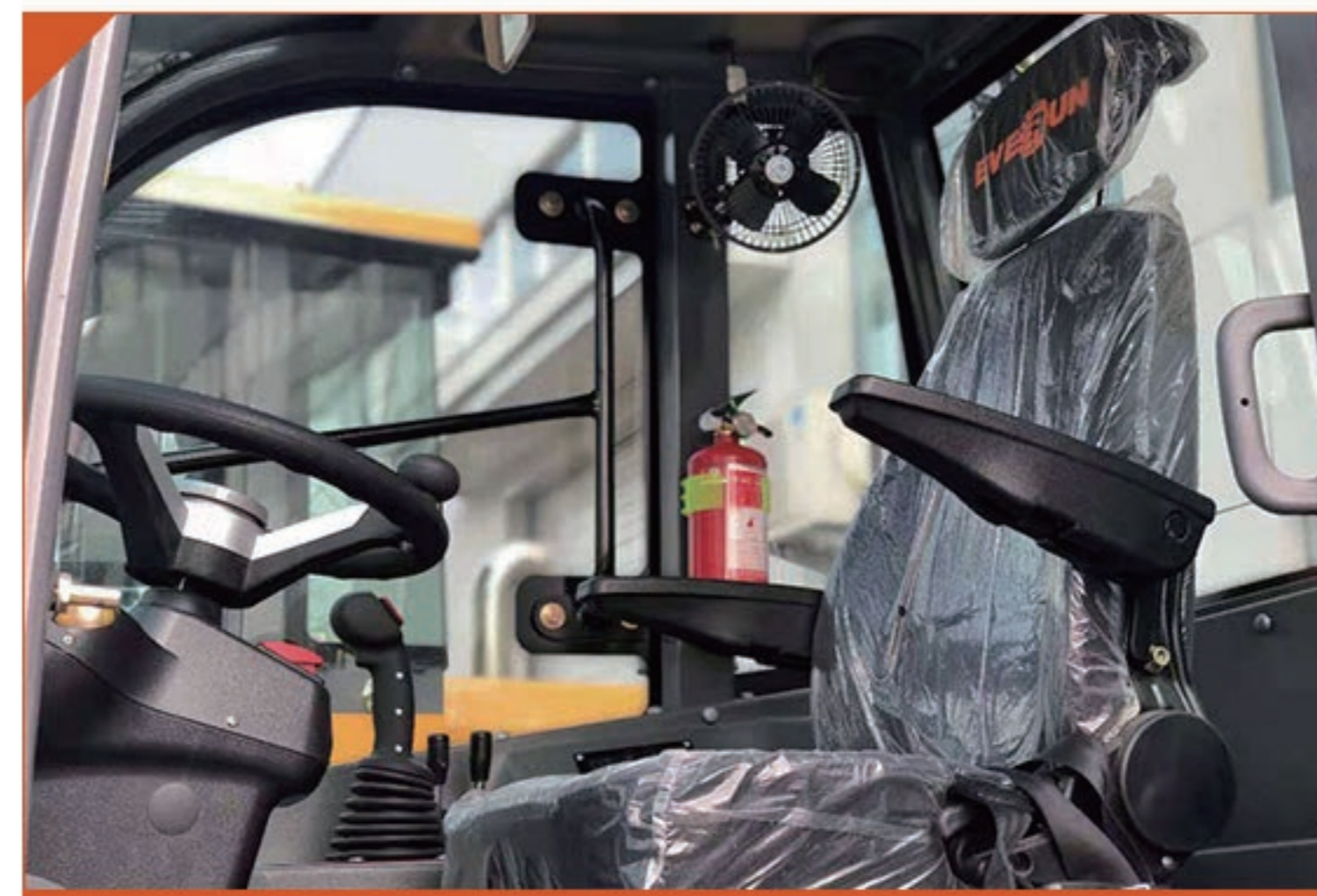
• ROPS & FOPS cabin with maintenance port
