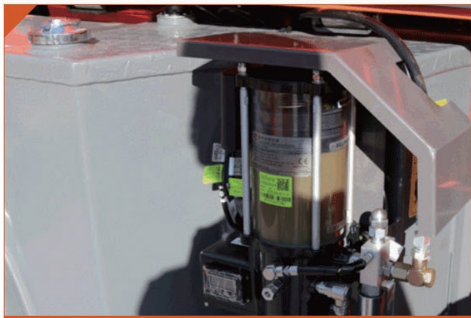
• Easily accessible lubrication points
